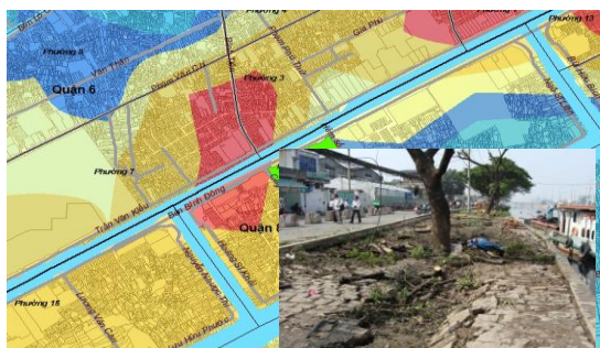
Figure 7. The substantial damage and time series of subsidence at PS (1996 – 2010)
